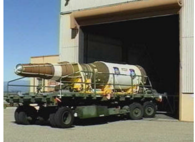
AltAir on Palletized Extraction System
